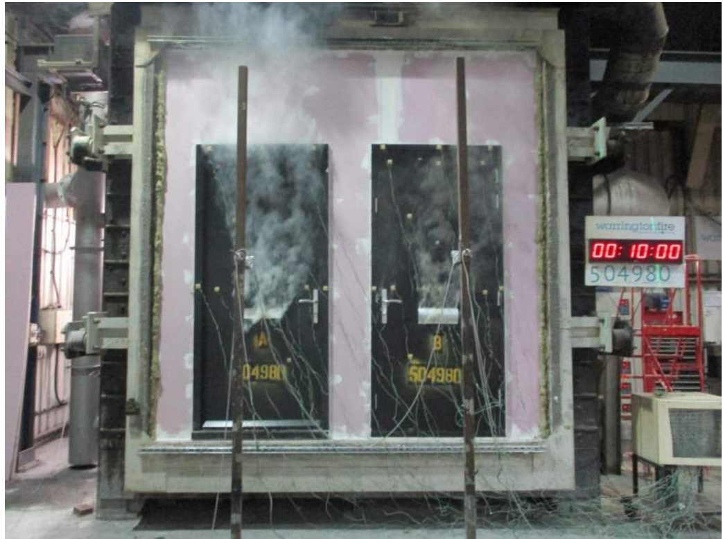
The unexposed face of the doorsets after a test duration of 10 minutes
