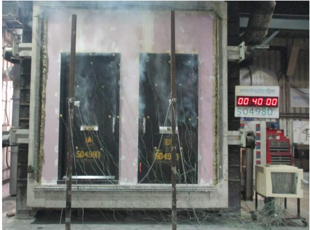
The unexposed face of the doorsets after a test duration of 40 minutes
