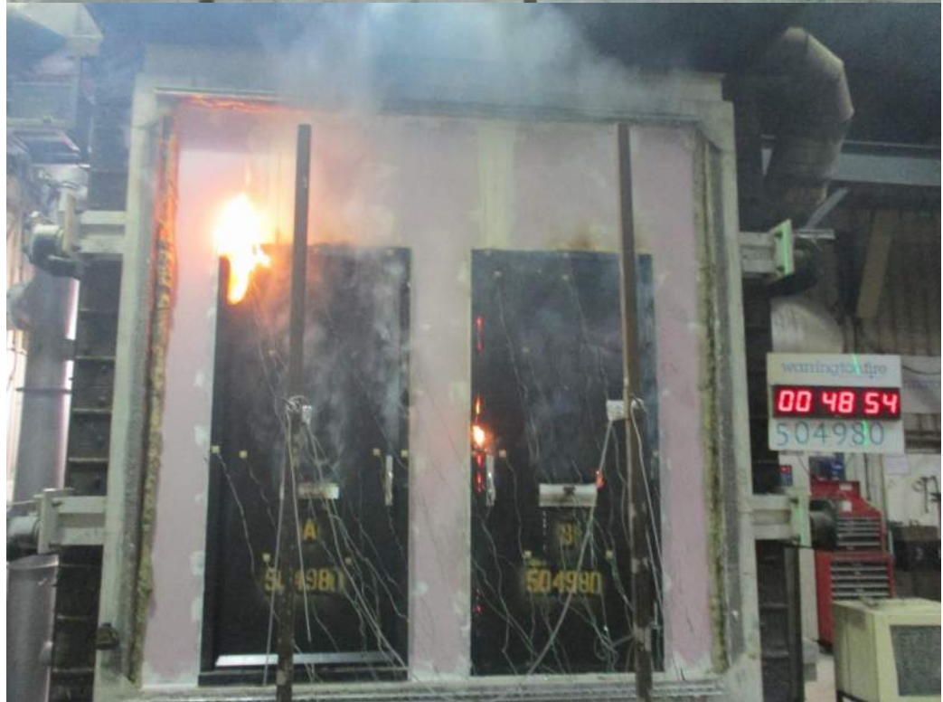
The unexposed face of the doorsets after a test duration of 48 minutes
