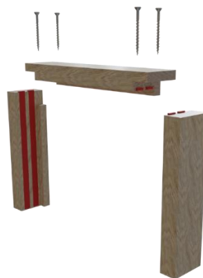
Trenched or Half Lapped Joint
