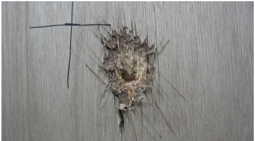
Damage to the sample following B.4.4.4 Manual cutting test
