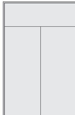
Double leaf Storey Height Door Assemblies with Flush Overpanel
