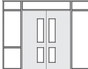
All timber must be straight grained, joinery quality free from knots, splits & checks. Minimum 70mm x 32mm (Min. density = 510kg/m³). This timber section can be used for both door frame jambs and transoms rails including within screens and for the perimeter framing for the screen and transom (fanlight).
